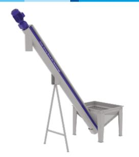
The crusher elevator is designed to carry the clean olives from the washing to the crusher mounted on the malaxer. It works automatically depending on the control panel and does not require operator intervention. In case of overloading the crusher automatically stops and prevents jamming of the crusher. It is made of stainless steel.
