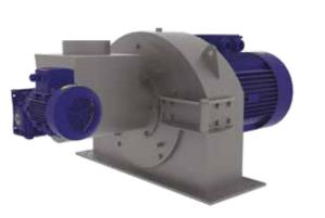
Clean olives coming from the washing machine with the crusher elevator are poured into the crusher feeding chamber and transferred from the center of the crusher to the crusher. In a fixed sieve, the hammers coupled to the motor shaft rotate at high speed, allowing the olives to pass through the holes of the sieve in small pieces and turn them into olive paste.
